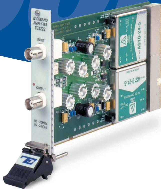
Model 3222 Is a 3U single-slot, PXI-based power amplifier designed for signal amplification. Offering unmatched signal purity, Model 3222 amplifies signals from dc to over 20 MHz. The unit has a fixed gain of x10, however, the same amplifier is available with custom gain, with no signal purity or performance degradation.
